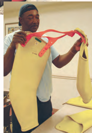
Lineworkers Roddy Bowers, left, Steve Ellerbe, top right, and Jimmie Ridges check their rubber insulated gloves and sleeves for any defects.
